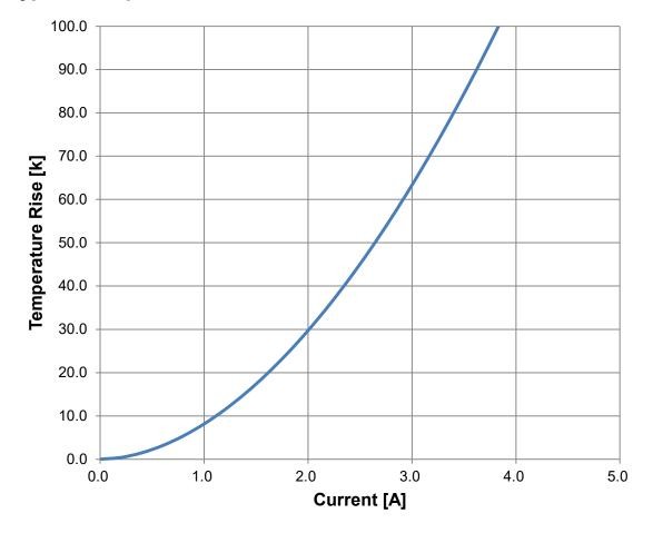
**Typical Temperature Rise vs. Current Characteristics**
