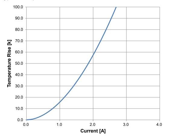
**Typical Temperature Rise vs. Current Characteristics**
