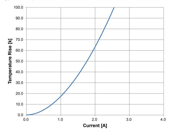
**Typical Temperature Rise vs. Current Characteristics**
